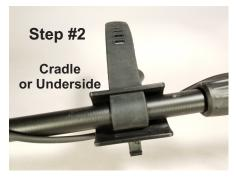
**Step #2** Lay the detector rod into the cradle side of the part you are going to attach as shown in the picture to the left. Thread the strap through the single slot side, pull it out through the front of the part pulling it away from you as shown in the picture Step #2. Attach Part B closet to the coil. Attach Part D closest to you.
